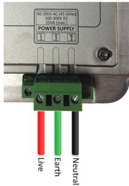
Figure 7: VECTO 3 power supply connection
