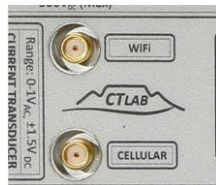
Figure 20: WiFi and Cellular Modem Connections
