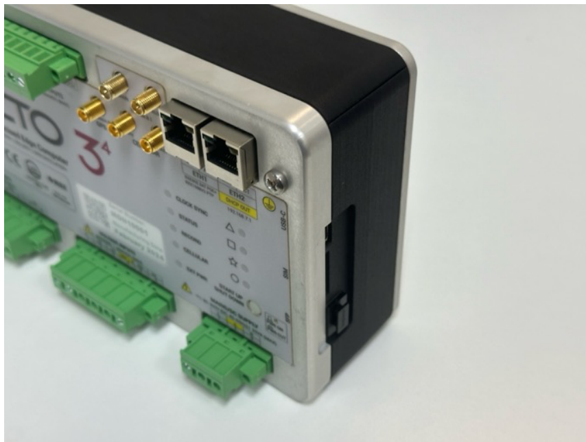
Figure 16: SFP cage with dust cover, SIM Slot and USB-C port
